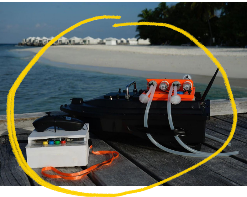
Here is one of the inventions I helped create called ATOMM, or Aquatic Trace Organism Molecular Monitor . It is used to safely collect eDNA from sharks without harming them! Each time the shark moves through its environment, it leaves behind a small trace of itself that I'm able to collect with ATOMM. This means that within a single scoop of water, I can get a sample of all the sharks that came through there that day! Credit: Gibbs Kuguru
